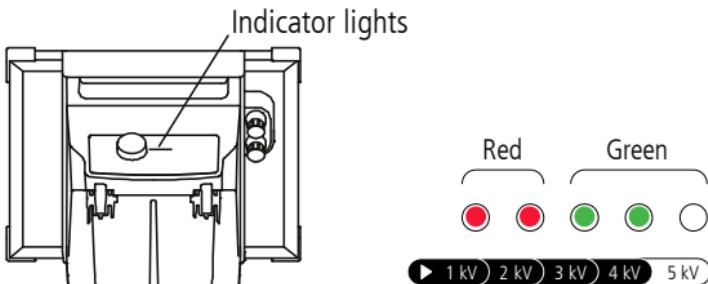
When first connected to the battery (and the Selector switch is set off), all the indicator lights illuminate for a period of two seconds. Thereafter, if any other switch positions are selected, the indicator lights display the output voltage at each pulse. This indicates that the energizer is operating normally.
